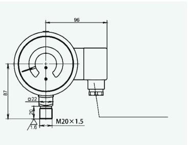
General radial type with right connection 普通径向型右出线
