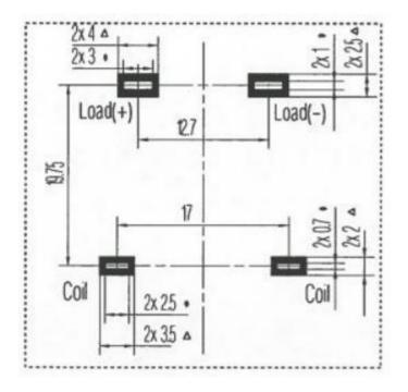
Note: The dimensions of \* is the opening dimensions of PCB board.
