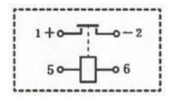
Note 1: No polarity on the coil, but polarity on the load.
